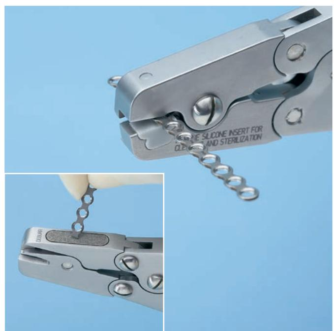
Plates 1.5 mm thick and larger can be cut using two short-cuts. A manual deburring feature is provided in the handle of each cutter if deburring is desired.
