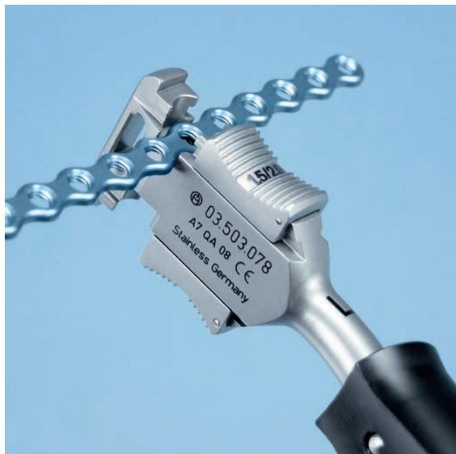
Keeping the handles in-plane, make the desired in-plane bend.
