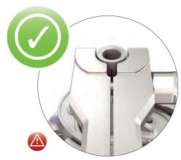
Slide the Offset Stabilizer Arm forward and tighten on to the Offset Adaptor by rotating the Offset Stabilizer Arm Locking Knob clockwise. Ensure that the black mark is aligned in the alignment window.
