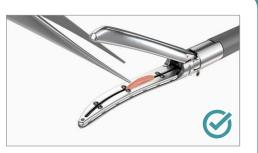
Do not clean instrument with abrasives If tissue is still visible in the jaws, use forceps to remove any residue taking care not to actuate the instrument.
